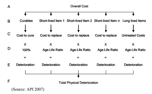
Figure 2. Age-Life Procedure for Estimating All Items of Physical Deterioration
