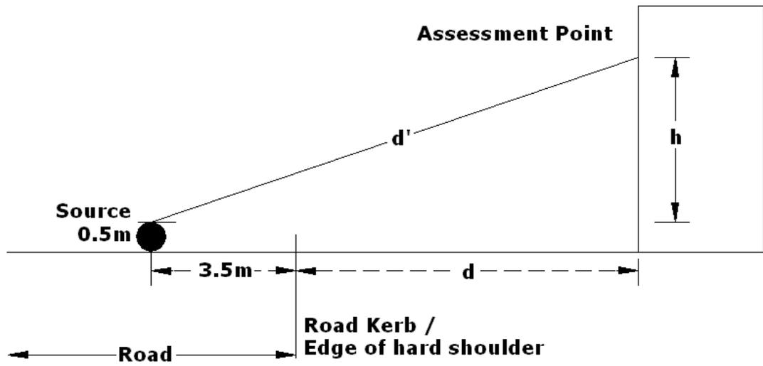
**Figure 2** Illustration of the shortest slant distance  $d'$  and the shortest horizontal distance  $d$  for a reception at a relative height  $h$  from the source line
